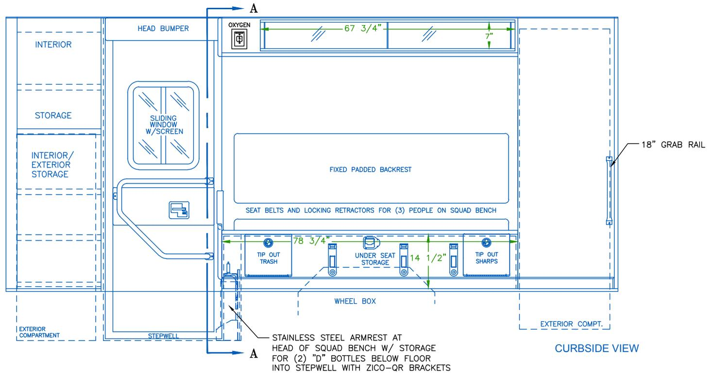
STAINLESS STEEL ARMREST AT HEAD OF SQUAD BENCH W/ STORAGE FOR (2) "D" BOTTLES BELOW FLOOR INTO STEPWELL WITH ZICO-QR BRACKETS
